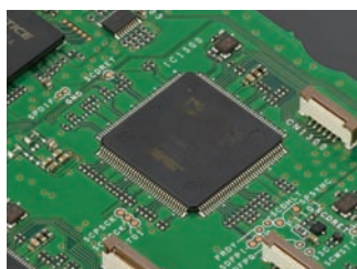
For band scope ADSP-21363 clock @332MHz
